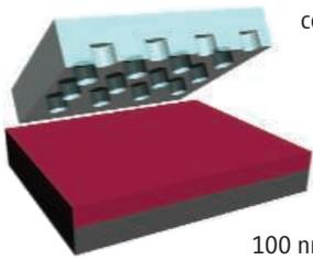
transmission and collimation of light through a subwavelength aperture.
