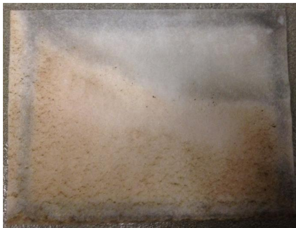
Example of what a spent filter pad looks like. This particular one was in use for 5 weeks.
